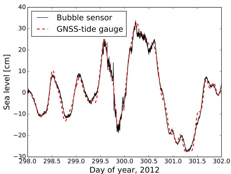
Figure 2 : Measurements from the bubble tide gauge at Onsala Space Observatory and the B-spline solution from the inversion algorithm.
